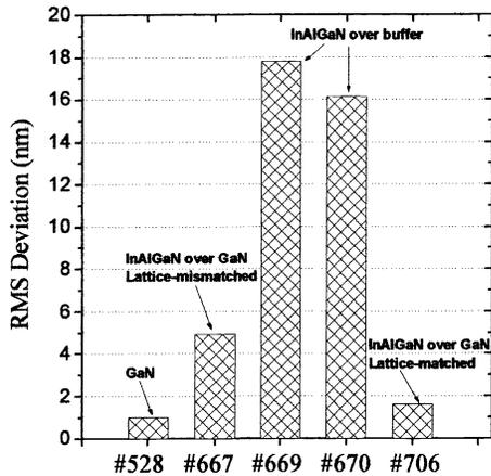
Figure 2(b). Atomic force microscopy (AFM) values of root-mean-square (rms) deviations of surface morphology of InAlGaN alloys. Sample #706 ( $\text{In}_{0.026}\text{Al}_{0.124}\text{Ga}_{0.85}\text{N}$ ) grown over GaN and lattice-matched with GaN has a smallest rms value comparable to that of GaN.
