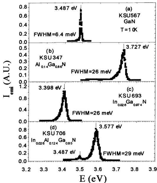
Figure 3. PL spectra of GaN, AlGaIn, InGaIn, and InAlGaIn measured at 10 K. We can achieve not only higher emission energies but also higher emission efficiencies in the UV region in InAlGaIn quaternaries than that in GaN. The emission efficiency of the InAlGaIn epilayers is also higher than that of the AlGaIn epilayer and is comparable to that of the InGaIn epilayer.
