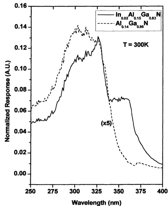
Figure 7. The response of  $\text{In}_x\text{Al}_y\text{Ga}_{1-x-y}\text{N}$  quaternary alloy (solid line) and  $\text{Al}_y\text{Ga}_{1-y}\text{N}$  ternary alloy (dotted line) with comparable cut-off wavelength. The compositions for these samples are estimated to be  $\text{In}_{0.02}\text{Al}_{0.15}\text{Ga}_{0.83}\text{N}$  and  $\text{Al}_{0.14}\text{Ga}_{0.86}\text{N}$ , respectively.
