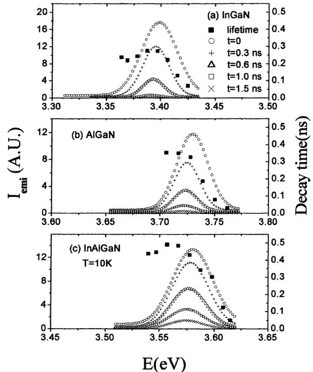
Figure 5. Time-resolved PL spectra as well as emission energy dependence of decay lifetime measured at 10 K for (a)  $\text{In}_x\text{Ga}_{1-x}\text{N}$  alloys, (b)  $\text{Al}_x\text{Ga}_{1-x}\text{N}$  alloys, and (c)  $\text{In}_x\text{Al}_y\text{Ga}_{1-x-y}\text{N}$  quaternary alloys.
