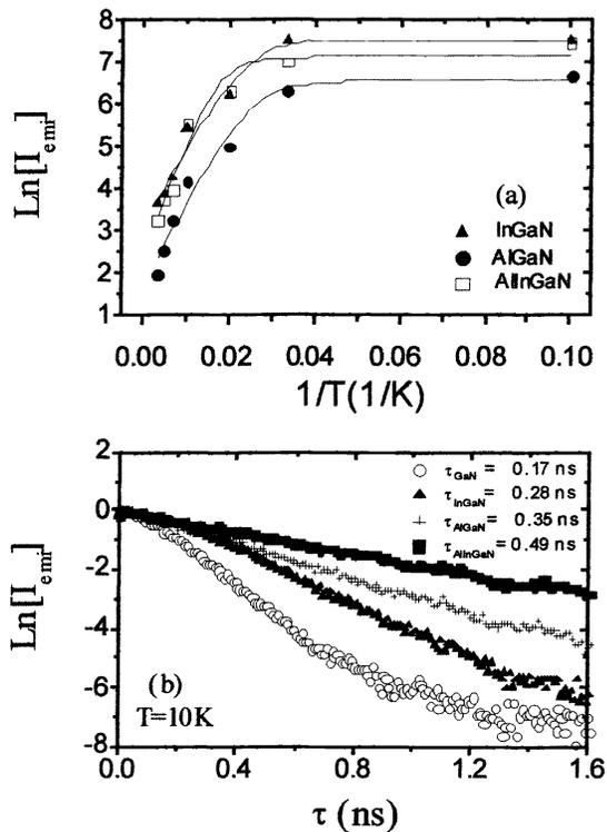
Figure 4 (a) The Arrhenius plots of PL emission intensities of InAlGaN, InGaN, and AlGaN alloys. (b) PL decay profile of InAlGaN quaternary alloy together with those of GaN epilayers, InGaN, and AlGaN alloys measured at T=10 K.
