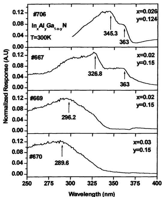
Figure 6. Normalized photoresponse versus wavelength of incident light of  $\text{In}_x\text{Al}_y\text{Ga}_{1-x-y}\text{N}$  quaternary alloys with different In and Al contents. The arrows indicate the cut-off wavelength for the quaternary alloys. The photoresponse from the underlying GaN epilayer in the two samples #706 and #667 is seen in the steps at 363 nm.
