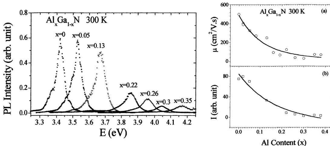
Figure 1. (Left) PL Spectra of  $\text{Al}_x\text{Ga}_{1-x}\text{N}$  measured at 300 K. (Right) Electron mobility and integrated PL emission intensity vs Al content measured at 300 K. The results show that both the emission intensity and the electron mobility of  $\text{Al}_x\text{Ga}_{1-x}\text{N}$  decrease exponentially with  $x$  - a potential problem for  $\text{Al}_x\text{Ga}_{1-x}\text{N}$  as active media for UV optoelectronic devices.
