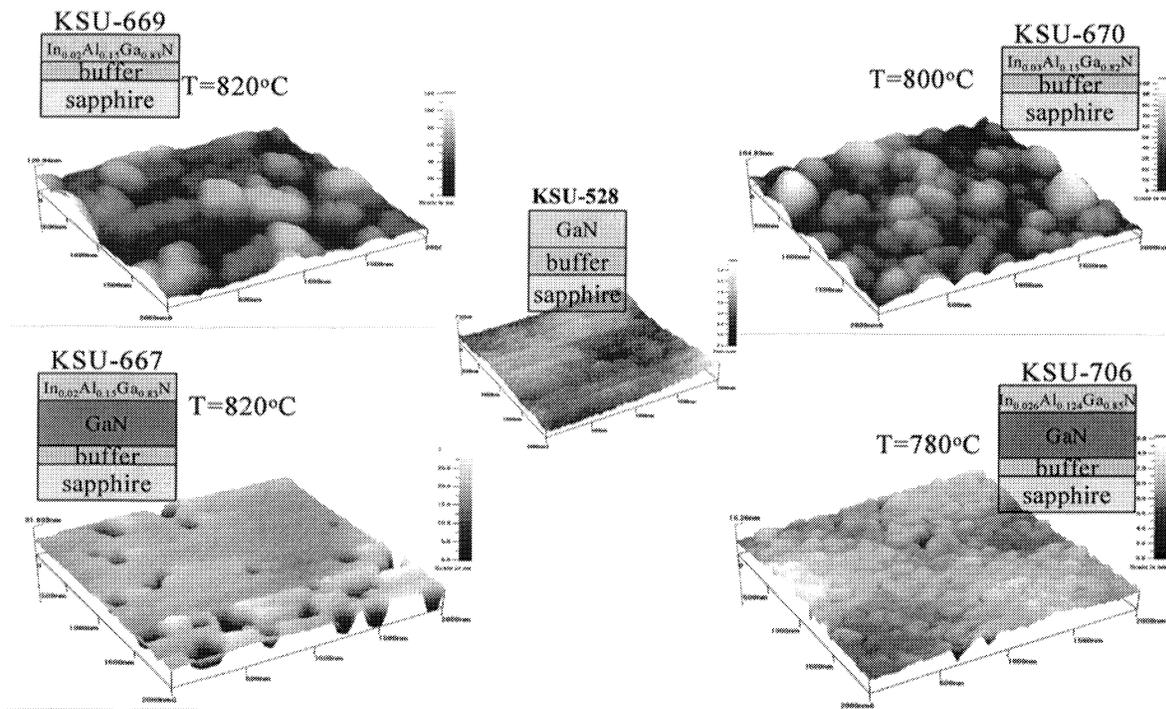
Figure 2(a) Atomic force microscopy (AFM) images (2 µm x 2 µm scan) for four InAlGaIn quaternary samples of varying structures and a GaN epilayer.
